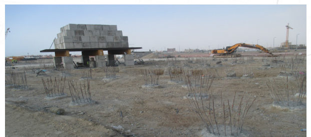
Pile Load Test - Building 843
